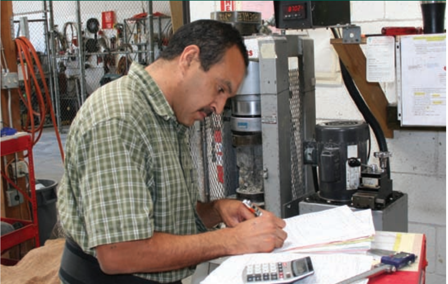
Alfonso Arellano, Assistant Laboratory Supervisor, Southwest Inspection and Testing Laboratory, recording the results from a concrete compression test.
