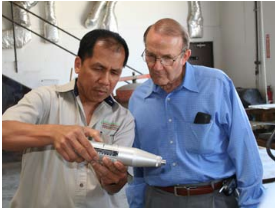
Renan Cruz, P. E., Quality Control Laboratory Manager with Southwest shows Roy Fewell a spring-driven steel rebound test hammer used to determine the compressive strength of in situ hardened concrete per ASTM 805.
