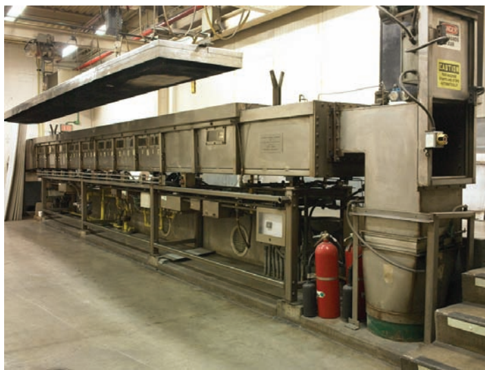
FIGURE 7-3 ASTM E84 test apparatus for measuring material's flame spread and smoke development indexes (Courtesy of Underwriter's Laboratories, Northbrook IL)
