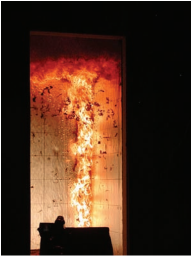
FIGURE 7-5 A room corner fire test of a wall and ceiling finish material
