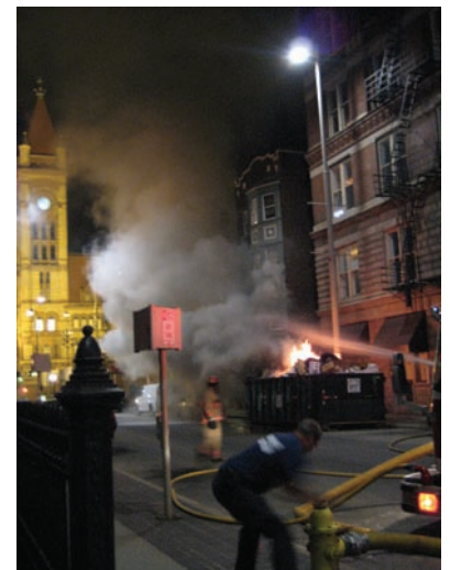
FIGURE 3-2 The IFC requires separation of outdoor dumpsters from buildings to limit the likelihood of the dumpster igniting an exposure building
