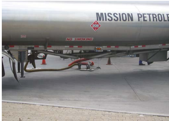
FIGURE 13-5 Connections from a tank vehicle to a storage tank must be liquid and vapor tight.
