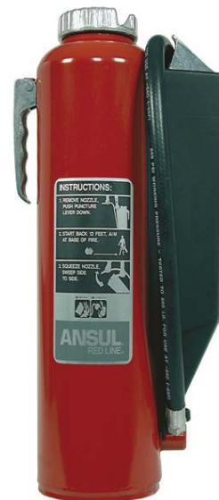
FIGURE 13-7 Portable fire extinguishers serving dispensers, pumps and tank fill connections require a minimum 20-B Class B fire hazard rating. (Courtesy of TYCO/ Ansul, Marinette, WI)
