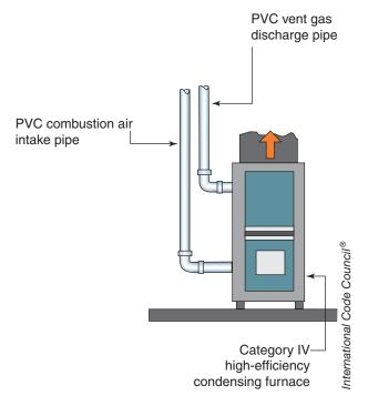
The sizing of plastic pipe venting material for Category II, III and IV appliances must be in accordance with the manufacturers' instructions.
