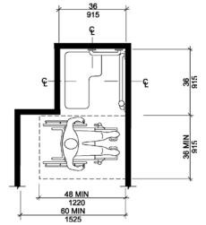
so the back of the person in the transfer space is lined up with the back wall of the shower seat. This will facilitate transfer from the chair to the seat and back. A common mistake is to place walls at both ends of the transfer space to form a type of privacy or dress-
