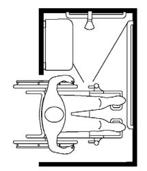
For an alternate roll-in shower, the transfer space is partially in the shower stall and partially through the stall opening. This allows for the same as the transfer from outside the transfer shower, or for someone to turn 90 degrees (instead of "parallel parking") and use the stall as a roll-in shower.
