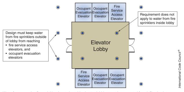
Water from operating fire sprinklers located outside elevator lobbies must be prevented from infiltrating into hoistways for fire service access elevators and occupant evacuation elevators.
