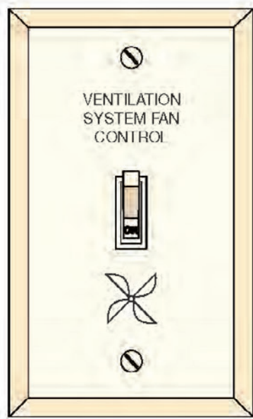
Labeling of controls for whole-house ventilation system
